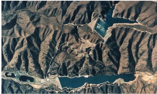
Figure 1.5: Aerial view of the Bath County Pumped Storage Power Plant's lower and upper reservoirs.
